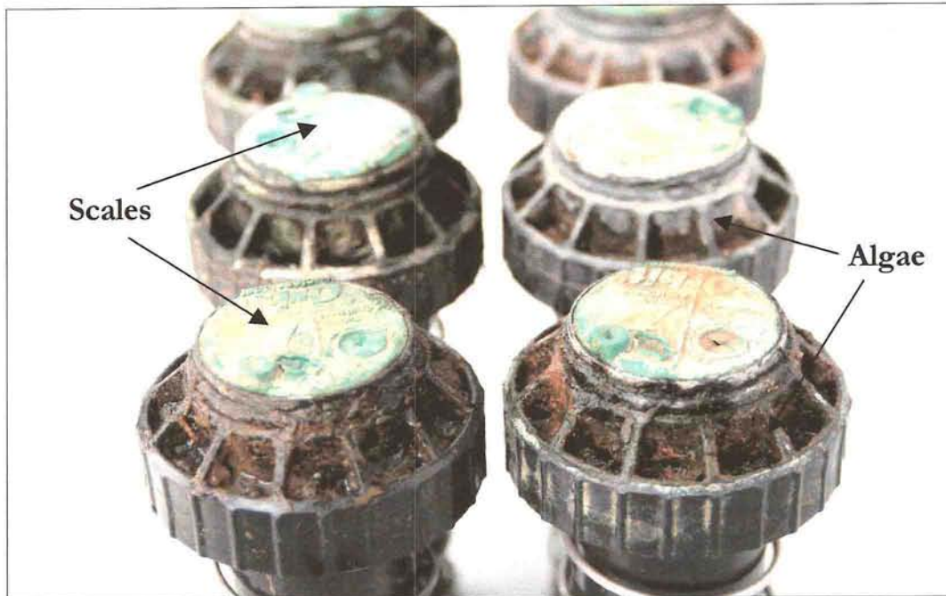
CONDITION OF SPRINKLERS AFTER 60 DAYS OF INSTALLATION (WITHOUT GMX)
